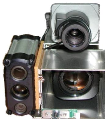
The unit can be mounted beside the camera system, pointing to the same direction. The unit will be set to triggering mode and triggering window defined to the desired distance.
