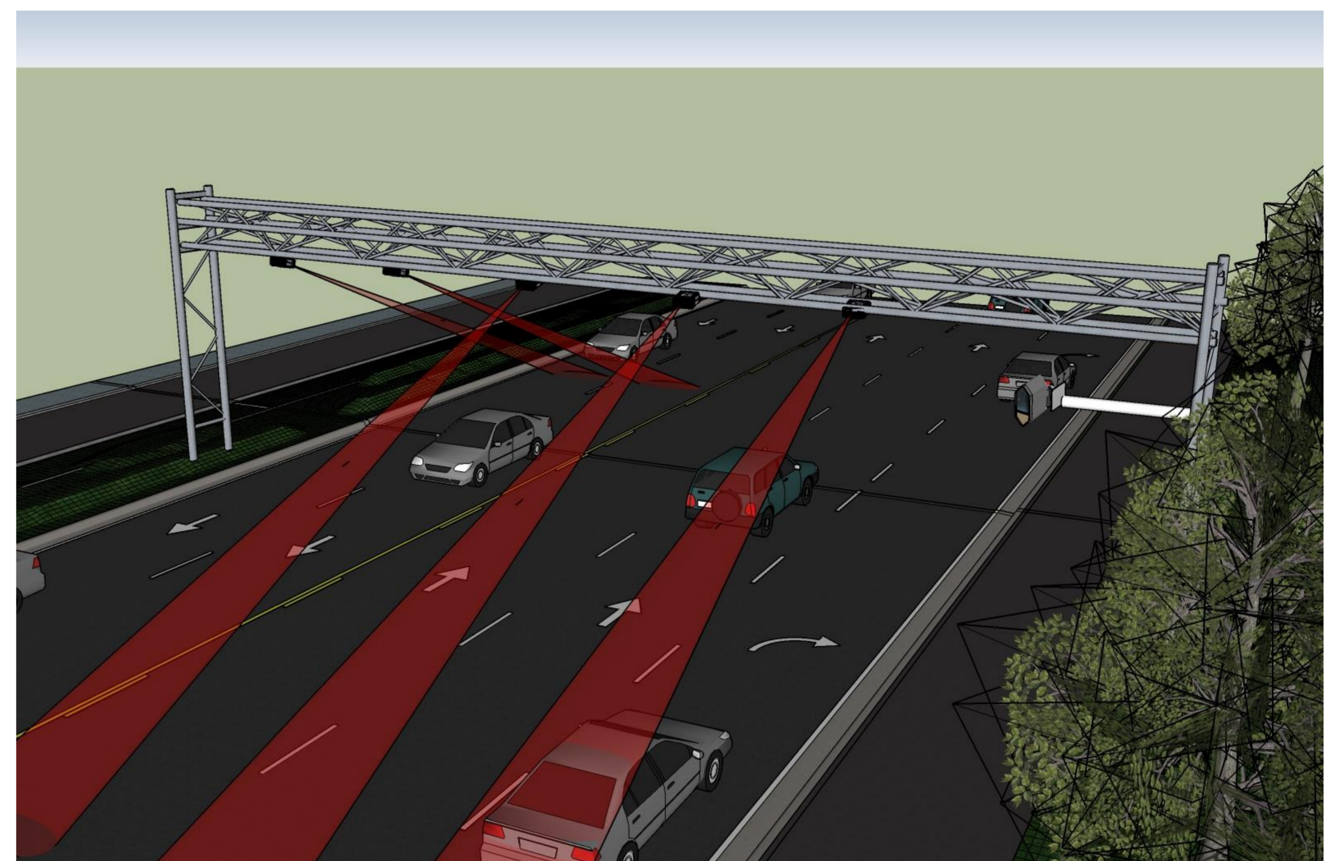
Road section monitored with Noptel sensors and Vidamin LPR-camera
