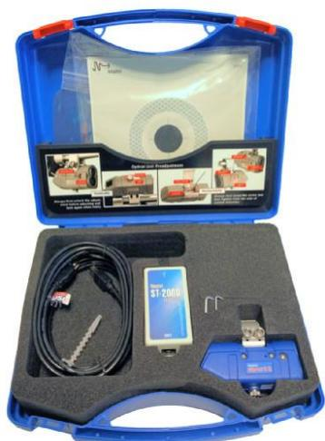
Noptel Sport II shooting training devices have been delivered since July 2003 and the same device type is still in production. Sport II device is connected to Windows PC by an USB-100 Box. It includes an USB-to-Serial converter that converts USB data transmission to standard RS-232 signals for Sport II device. For the USB converter to function correctly, a device driver is needed in the PC.
